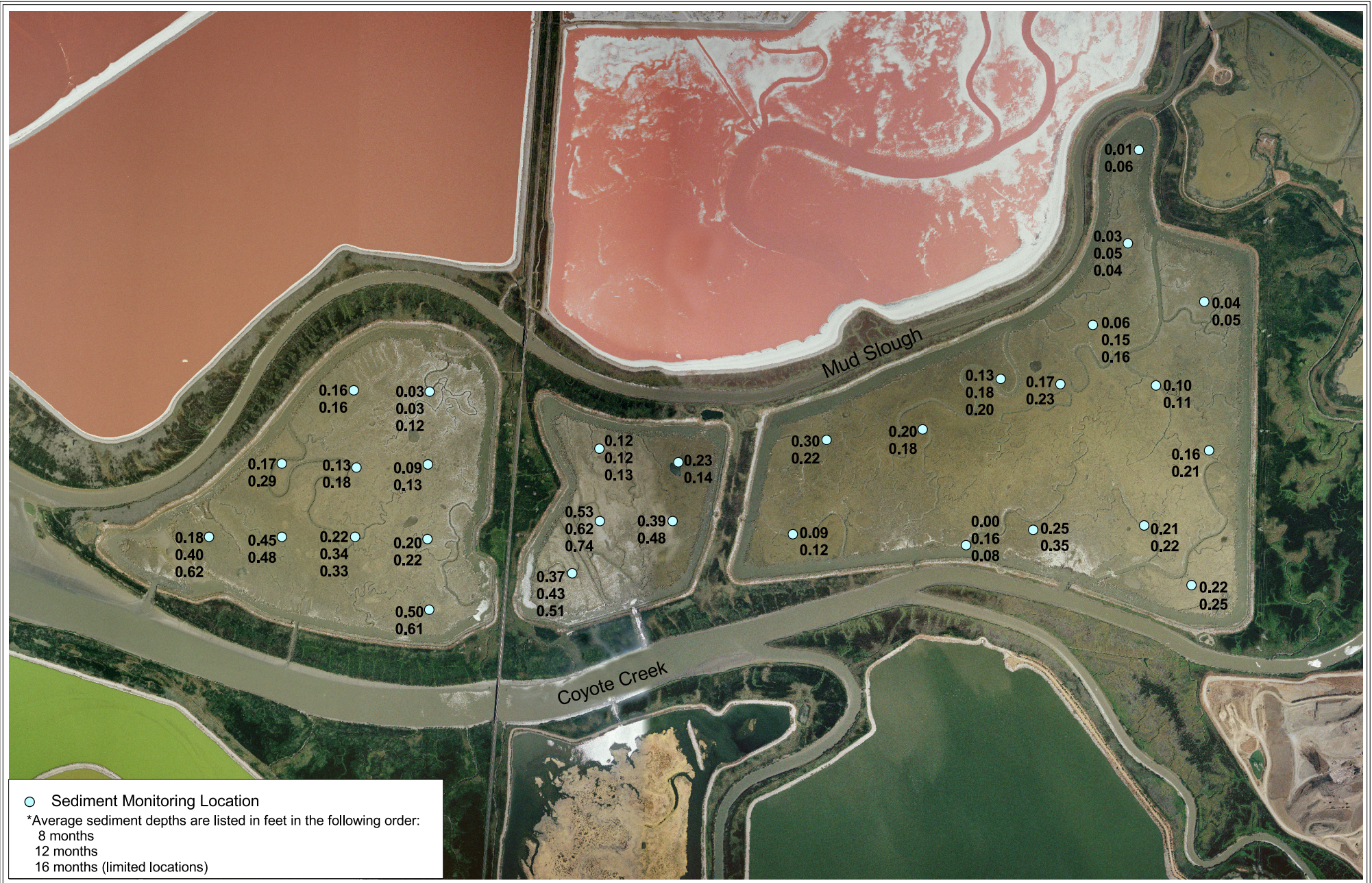
Figure 6. Island Ponds Sedimentation Data Average Sediment Depths 8, 12 and 16 Months Post-Breach
